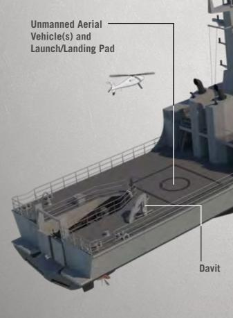
Long-endurance reconaissance Unmanned Aerial Vehicle launch and recovery system on aft deck.
